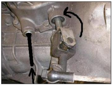
Stick drill of 5mm into the hole and turn to lock.
